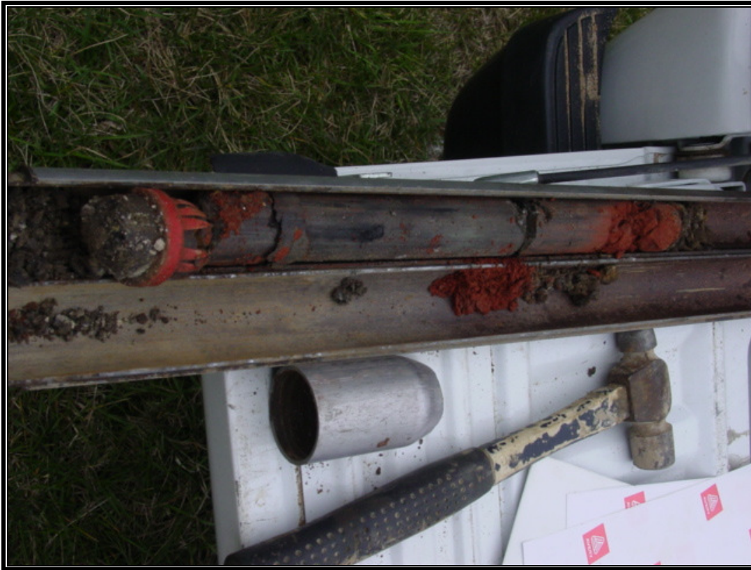
Figure 4.2. Example of a split spoon sample.
